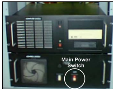
Figure 3-1: Main Power Switch
