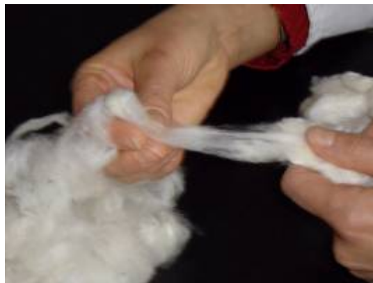
Figure 1: "Opening and mixing" a cotton sample by hand (Picture CIRAD, 2008).
