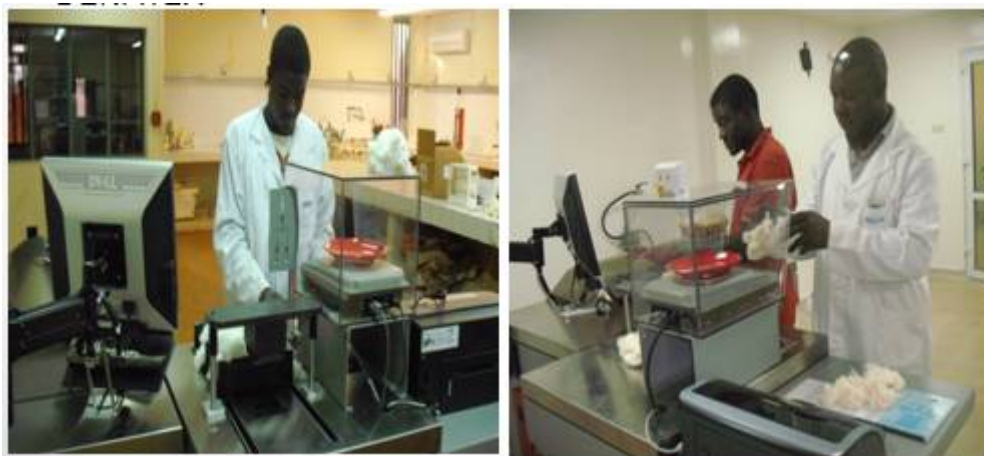
Instrument based cotton classing operation with the Uster HVI 1000 Integrated Testing Line
